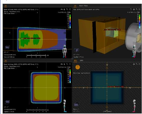
A simple geometry water phantom with a simple beam set and beam must be initially manually configured in RayStation. Square and circular apertures are automatically build to physical specifications as illustrated in the methods section.
