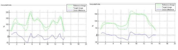
(I) Gamma Analysis: difference between planned and measured dose profiles
