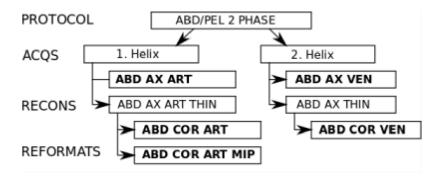
The Philips Brilliance scanners add another layer to the hierarchy: the "Reformat". Sagittals, coronals, oblique, and MIP series are all Reformats and must be built from an axial series. The parent axial series are generally "thin" (<1mm thick) to allow adequate resolution in the reformats, and need not be sent to PACS.
