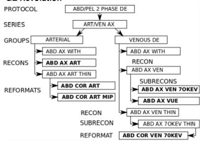
The Revolution user interface adds one more layer specific to dual energy protocols: the "Subrecon". Parameters like image thickness and interval are specified at the Recon level, and dual-energy recon parameters are specified at the Subrecon level.
