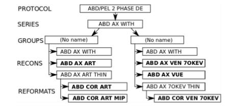
GE scanners using the Lightspeed user interface add another layer. Each acquisition is called a "Group", and the groups are combined into "Series". The first recon series in each group has the same name as the "Series" level. Another feature is that the reformats are
