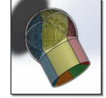
Schematic of the proposed high resolution 3D spherical detector. It would consist of 16 semispherical concentric layers, 31,560 isotropically distributed photodiodes and five active matrices per layer for detector readout.
