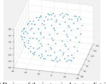
MathCAD view of the isotropic detector distribution within the 3D array
