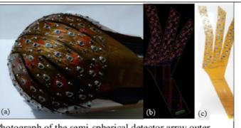
Photograph of the semi-spherical detector array outer layer (a). Active matrix design performed in Autodesk EAGLE software (Autodesk Inc, San Rafael, CA) (b). Active matrix made out PCB Flex (c).
