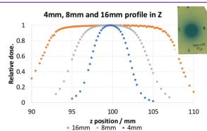
Left: Profile scans in z direction for irradiation with all 8 sectors set at the 4mm, 8mm and 16mm collimator using 4.0 the W2 scintillator. The table summarizes the FWHM and 3.5 the TMR10 prediction.
