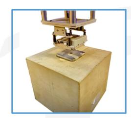
Set cutouts on top of solid water, with the top of the solid water set to 100 cm SSD. A standard 6x6 cm<sup>2</sup> applicator was placed in the LINAC head.
