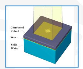
Simulated electron irradiation setup using RayStation's electron Monte Carlo. Each cutout and bolus combination was simulated with 5 million histories.
