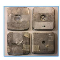
Poured cerrobend cutouts with holes of 10, 15, 20, and 30 mm (nominal diameter). Cut 5- and 10-mm thick bolus to fit holes. Placed 1.5 mm of beeswax underneath cutouts to reduce hotspots.
