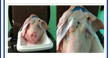
Accelerometers were attached on the hog head on the distal side of the proton beam. The detected acoustic signal was overlapped with proton pulse and simulation, in which the acoustic TOF agrees with the distances between BP and detector calculated
