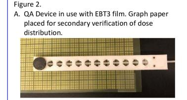
B. Film post QA. Note shadowing indicating distance of seed. Profile provides a digital measure of brass pin placement relative to set seed position.
