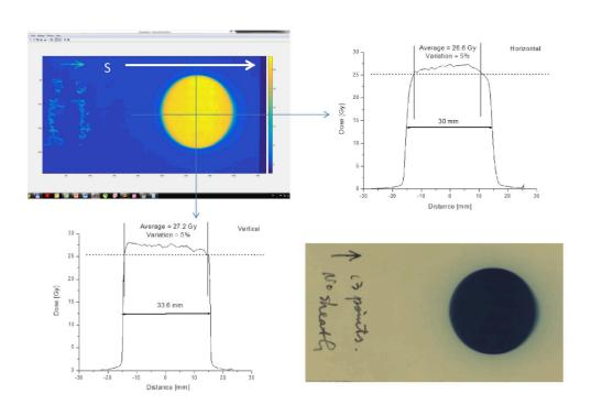
Figure 1: Results of dose distribution measurements around novel 50 kVp rectal applicator: 2D dose distribution (up-left); horizontal dose profile (up-right); vertical dose profile (bottom-left); measurement film piece (bottom right).
