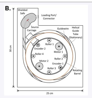
Figure 1: (a) Simplified block diagram of the modular remote afterloader (MRA). (b) MRA cartridge containing the guidewire-mounted radiation source, the shielded safe, and the quidewire drive system. The helical guide tube has three 360° wrappings.
