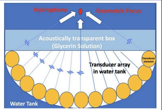
The experimental setup is shown in the figure. The transducer contains 112, 500 kHz elements with transmit and receive capabilities. A polycarbonate box was fabricated with acoustically transparent film to hold a glycerin solution for which the speed of sound is closely matched with that of the human skin. The hydrophone to measure pressure is placed at the geometric focus during the experimental validation.
