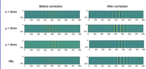
The figure shows pressure field maps from the transducer used to gather the experimental data at different distances from the geometric focus. The pressure that is regained as a result of aberration correction can be visualized. The distance scales of the axes are in arbitrary units.
