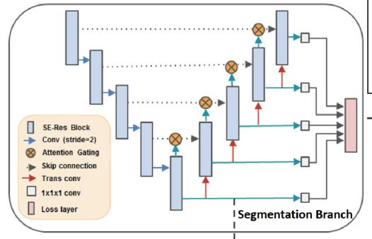
The architecture of the proposed segmentation model, which is implemented with PyTorch with GPU acceleration. Note that only segmentation branch will be used for model inference while the classification branch will be included into model training.
