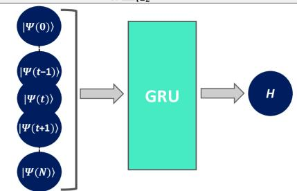
Flow of information through the RNN for the quantum model. States were fed into a Gated Recurrent Unit (GRU) neural network to predict the parameters of H.
