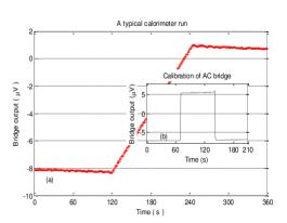
Typical irradiation run obtained using the NIM 6MV photon beams in (a), the uncorrected voltage signal was 9.377 μV and the water temperature was 3.983 °C measured by three Pt-100 probes. The response to a 1 Ω increase in the decade box resistance is shown in (b), the uncorrected voltage signal was 12.801 μV, and the water temperature was 4.059 °C.
