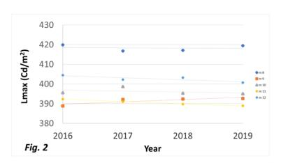
Figures 1,2 and 3 present the results of annual measurements of the maximum luminance ( $L_{max}$ ) in years: 2016-2019. All monitors are automatically calibrated for  $L_{max}$ = 400 cd/m<sup>2</sup>. Six monitors out of 18, showed an increase of  $L_{max}$  during the tested period of four years (Fig.1). Five monitors did not show any statistically significant change of  $L_{max}$  (Fig. 2) and 7 monitors showed a decrease of  $L_{max}$ , during the period of four years (Fig.3).
