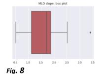
The plot on the left (Fig. 7) illustrates a distribution of  $r^2$ -scores for the MLD measurements. For the box plot on the right (Fig.8), we also restrict to a subset of monitors where the fit is good:  $r^2$ -score >= 0.5. The isolated point in this figure corresponds to an outlier monitor which has an MLD slope that is too steep compared to the other monitors.
